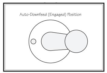
Figure 40. Downfeed selector in the auto-downfeed (engaged) position.
